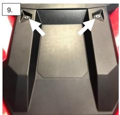
Re-torque all the fasteners after 100 miles.
